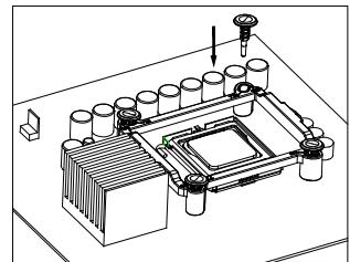
3. Insert four plastic pins into the hole of the plastic insert.
