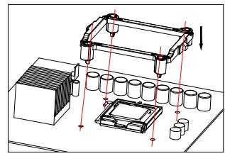
2. Install the mounting bracket on the motherboard and push the four plastic hooks through the mounting hole.
