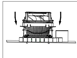
4. Install the cooler by pressing the mounting clip down until it's secured.
