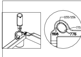
1. Install four plastic inserts into the hole of the mounting bracket according to your CPU socket type.
