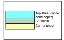
Label paper has a structure comprising of three layers, as shown in the diagram. The top sheet is printed on. The adhesive layer consists of pressure-sensitive adhesives. The carrier sheet (also called the linear or backing sheet) holds the labels until used. Due to the complexity of its composition, adhesive-backed label paper is particularly likely to give printing problems.
