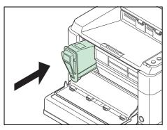
4 Install the new toner container in the printer. Push in firmly until you hear a "click" sound.
