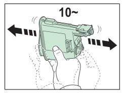
3 Take the new toner container out of the toner kit. Shake the new toner container at least 10 times as shown in the figure in order to distribute the toner evenly inside the container.
